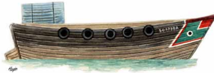
Figure 2: Drawing of a traditional cargo barge operated by ethnic Chinese in Singapore and Malaysia from the 19th century until the end of the 20th century, when the type was made obsolete by the introduction of container ports. Known by the local Malay name of tongkang , the bows of these barges are painted with colourful patterns that invariably include a pair of eyes. The practical rationale of these bow patterns is a safety measure in the crowded waterways by rendering the boat more conspicuous and its direction of travel more obvious. (Original drawing by Lee Ho Yin)
